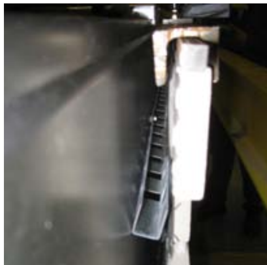
Figure 1. Vertical load arrangement. Figure 2. Loaded with dead weight + 120 kg.
