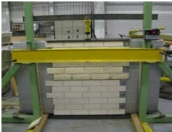
Figure 1. Vertical load arrangement. Figure 2. Loaded with dead weight + 120 kg.
